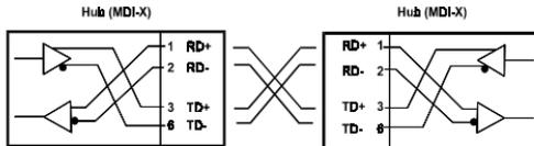
**Crossover cable for DSS-8+ (MDI-X port) to switch/hub or other network devices (MDI-X port) connection**
